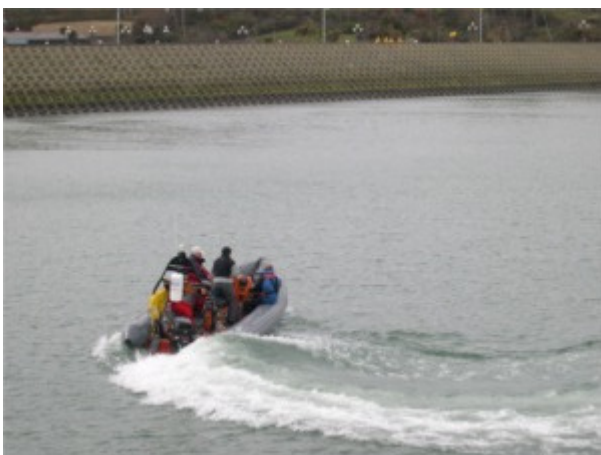
The rib is highly manoeuvrable as Greg encouraged us to find out. Due to the shape of the hull, it is possible to turn the boat at speed, as the ridges along the length of the boat grip the water.
